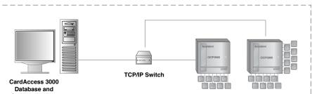
CICP2800 Eight/Sixteen Door intelligent Controller The Accelaterm can connect to the CardAccess Server via 10 /100 Base-T LAN/WAN (Standard), EIA-232 (Optional) and EIA485 (optional). Refer to the Accelaterm Service and Installation manual for additional detailed system wiring information.
