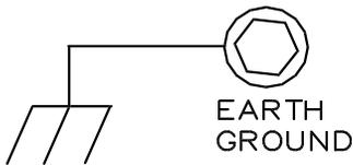
**NOTE:** Do not use a gas pipe, plastic pipe or AC ground connections.
