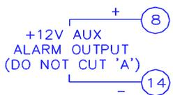
Auxiliary Output can be activated depending on the programming options selected (see GEM-P3200 Programming Instructions). Connect the device controlled by the programmable output between terminal 8 (+) and terminal 14 (-). A programming option "Aux. Output Chirp on Key-fob Arming" is available. If selected, an external siren driver can be connected to these terminals.
