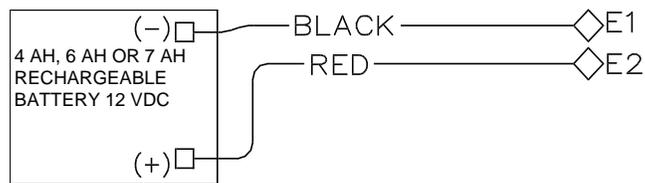
The RED (+) and BLACK (-) flying leads must be connected to a 12VDC 4, 6 or 7 AH Rechargeable Battery, to serve as backup power in the event of AC Power Failure. **NOTE:** To calculate the available standby time refer to the Standby-Battery Calculation Worksheet at the back of this manual.
