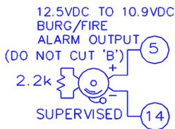
Connect the alarm sounding devices (self-contained sirens, speakers or a mechanical bells) to terminals 5 (+) and 14 (-). Any self-contained siren requiring a 12 VDC input can be connected. When connecting a mechanical bell, it must be supervised using a 2.2k Ohm resistor. To connect 8 Ohm Speakers use a Siren Driver with the proper polarity observed. **NOTE:** Refer to the Wiring Diagram for alarm current specification, bell supervision and burglary output relay.
