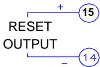
Reset Output can be activated depending on the programming options selected (see GEM-P3200 Programming Instructions). Connect the device controlled by the programmable output between terminal 15 (+) and terminal 14 (-).
