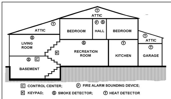
At least one smoke detector should be installed directly outside each sleeping area. If there is more than one floor, additional smoke detectors should be installed on each level, including the basement. The living-area and basement smoke detectors should be installed near the stairway of the next upper level.
