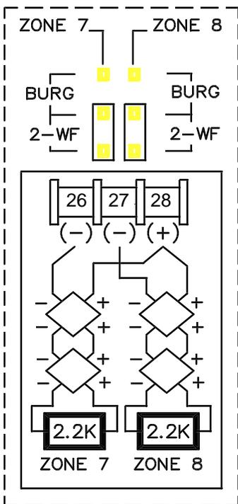
Two-wire smoke detectors can only be connected to zones 7 and 8. To use them, select fire zone programming option and select 2-wire smoke detector programming option for the desired fire zone 7 or 8 (refer to the GEM-P3200 Programming Instructions) and set JP7 to the position as shown. Connect the 2-wire smoke detectors as shown.
