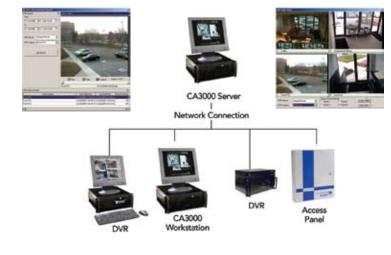
The CA3000 software communicates with any supported DVR Server on the network via TCI/IP protocol. All DVR servers are time-synchronized with the CA3000 Server. So no matter where the video is being stored, across the street or across the country, the CA3000 can find it.
