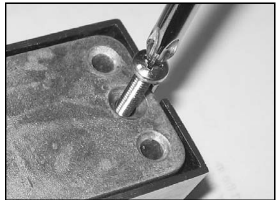
Fig. 5: The rear Phillips screw on the locks or unlocks the battery cover.
