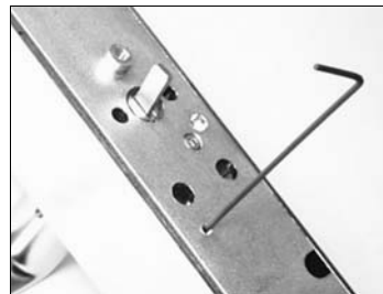
Fig. 1c: Use 1/16" hex wrench to screw in the cylinder back stop screw
