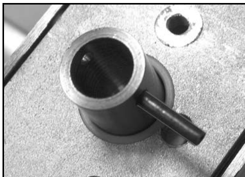
Fig. 4b: Insert Roll Pin into one Hub hole.
