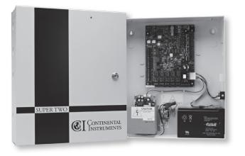
The two-reader Super-Two (CICP-1300) supports 2 readers and has 8 inputs, 1 tamper alarm and 5 relay outputs. A locking steel enclosure, power supply and 7AH battery are included. Plug-in network interface, memory expansion, X-Y matrix keypad support and input/output expansion are optional. In addition to power for the controller and two readers, 1.2A at 12VDC is provided for accessories, including power strikes and mag-locks.
