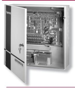
The eight-reader Superterm (CICP1800) supports 8 readers and has 24 inputs, 1 tamper alarm and 17 outputs. A locking steel enclosure, power supply and battery are included.
