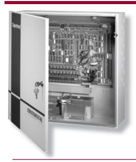
The four-reader Superterm (CICP1400UL) supports 4 readers and has 16 inputs, 1 tamper alarm and 9 outputs. A locking steel enclosure, power supply and battery are included.
