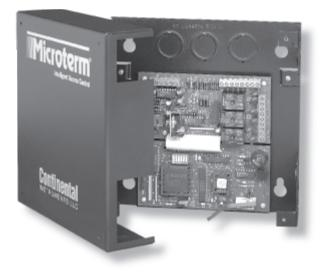
The Microterm (CICP1100) has 2 inputs, 1 tamper alarm and 3 outputs, and is housed in a steel enclosure.
